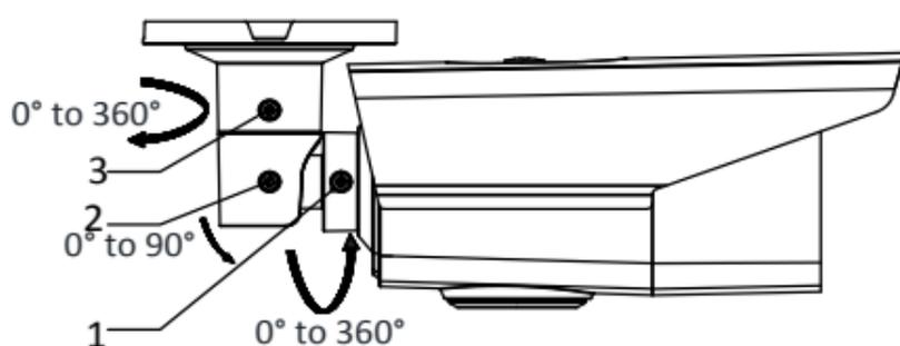
Figure 2. 3 3-Axis Adjustment
