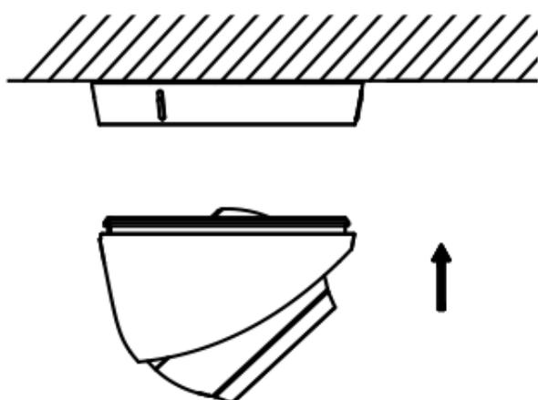
Figure 2. 7 Secure the Camera with Mounting Base
