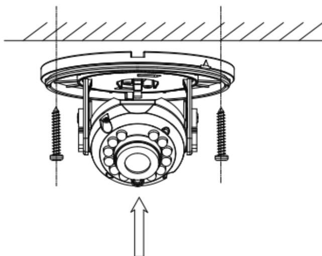
Figure 2. 11 Attach the Mounting Base to the Ceiling
