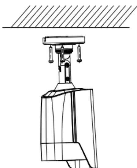
Figure 2. 2 Secure the camera to the ceiling
