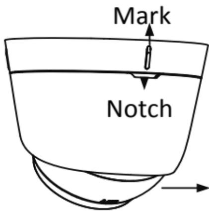
Figure 2. 4 Disassemble the Camera
