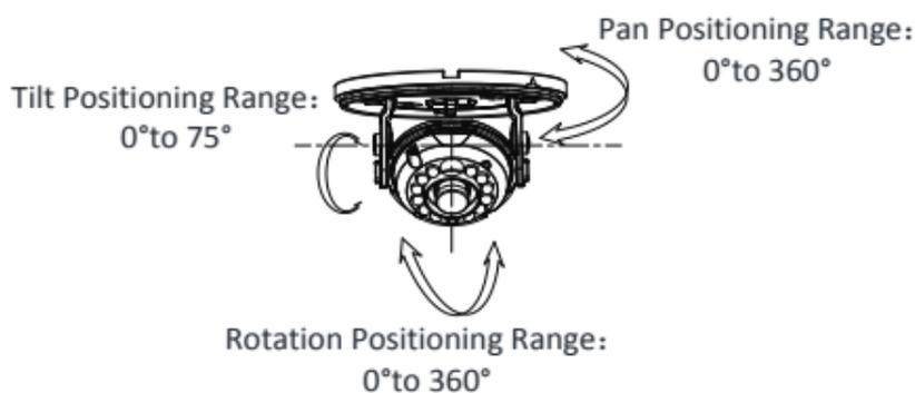
Figure 2. 12 3-axis Adjustment
