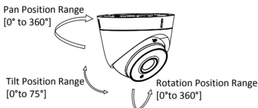
Figure 2. 8 3-axis Adjustment
