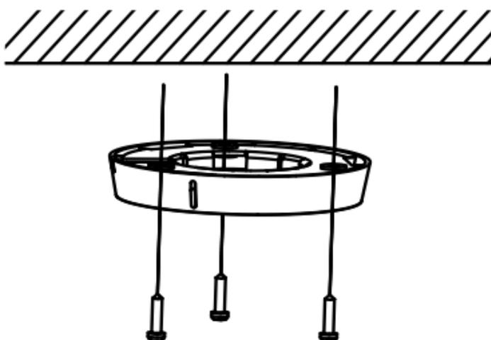
Figure 2. 6 Attach the Mounting Base to the Ceiling
