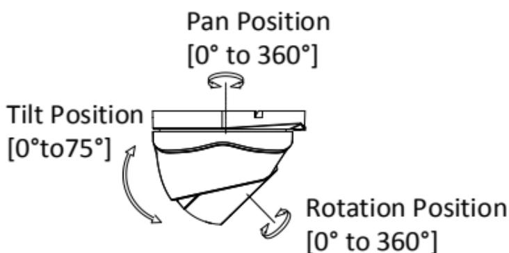
Figure 2-10 3-axis Adjustment
