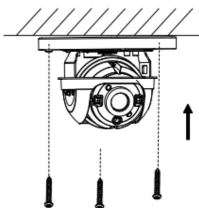
Figure 2-13 Fix the Mounting Base
