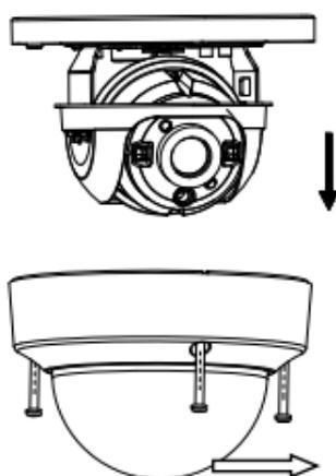
Figure 2-12 Remove the Bubble
