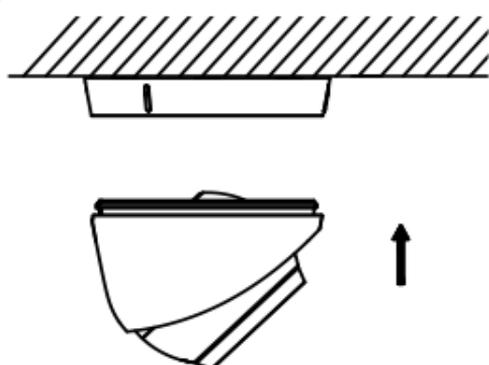
Figure 2-4 Secure the Camera with Mounting Base
