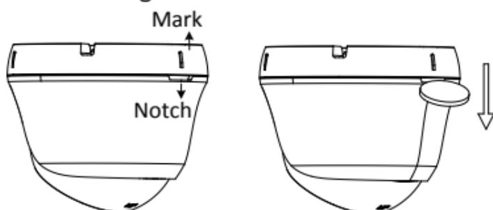
Figure 2-1 Disassemble the Camera
