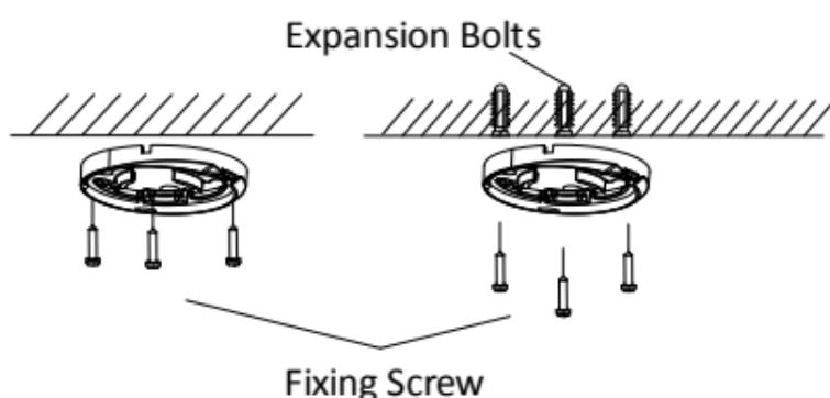
Figure 2-8 Fix the Mounting Base to the Ceiling
