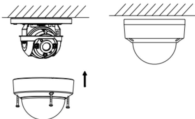
Figure 2-15 Bubble Reinstallation
