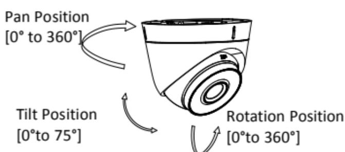
Figure 2-5 3-axis Adjustment
