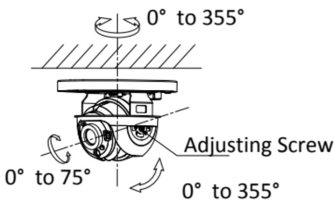
Figure 2-14 Type I Camera 2-Axis Adjustment
