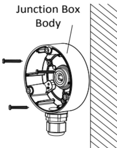
Figure 2-6 Secure Junction Box on Wall/Ceiling
