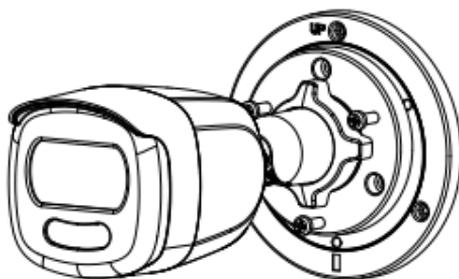
Figure 2-5 Attach Camera on Junction Box's Cover
