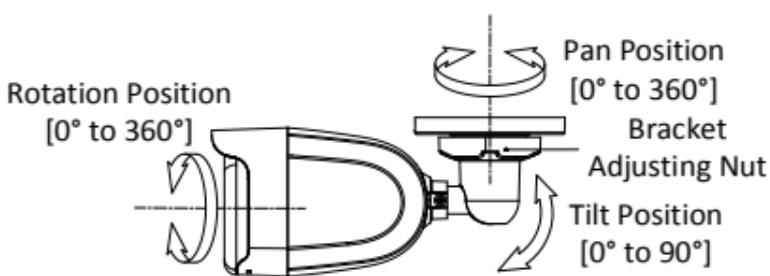
Figure 2-3 3-Axis Adjustment
