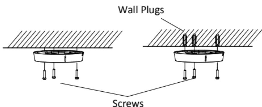
Figure 2-14 Attach Mounting Base to Ceiling
