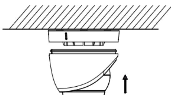
Figure 2-15 Install Camera Back
