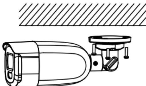
Figure 2-9 Secure the Camera to the Ceiling
