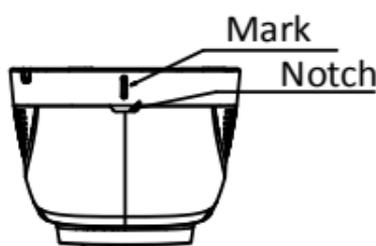
Figure 2-11 Disassemble Camera
