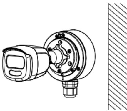
Figure 2-7 Combine Junction Box Cover back to its Body
