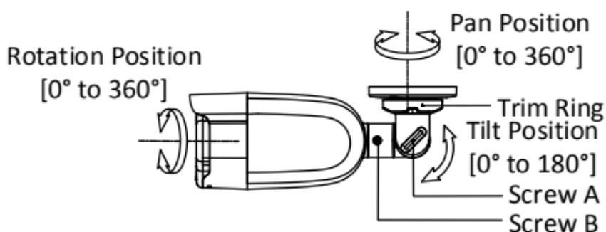
Figure 2-10 3-Axis Adjustment
