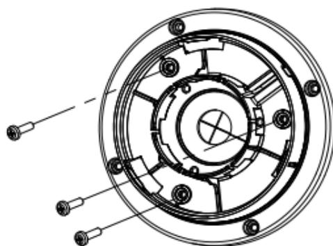
Figure 2-18 Secure Screws on Junction Box's Cover
