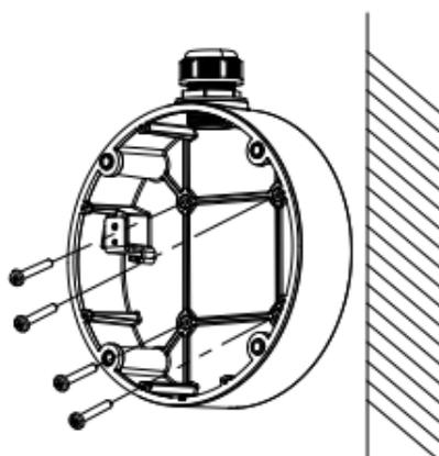
Figure 2-19 Secure Junction Box's Body
