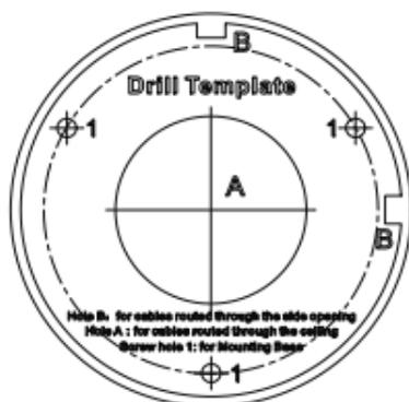
Figure 2-4 Drill Template of Junction Box
