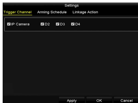
Figure 5. 17 Set Trigger Camera of VCA Alarm
