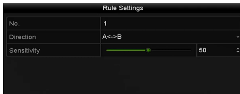
Figure 8. 13 Set Line Crossing Detection Rules
