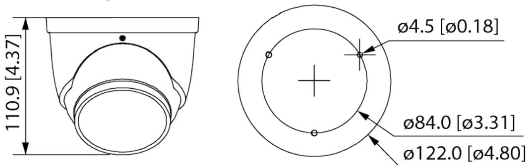
Figure 3-3 Dimensions: Model B (Unit: mm [inch])
