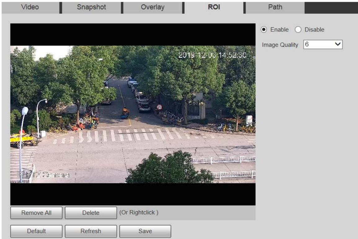
**Step 2** Select **Enable** to enable this function.
