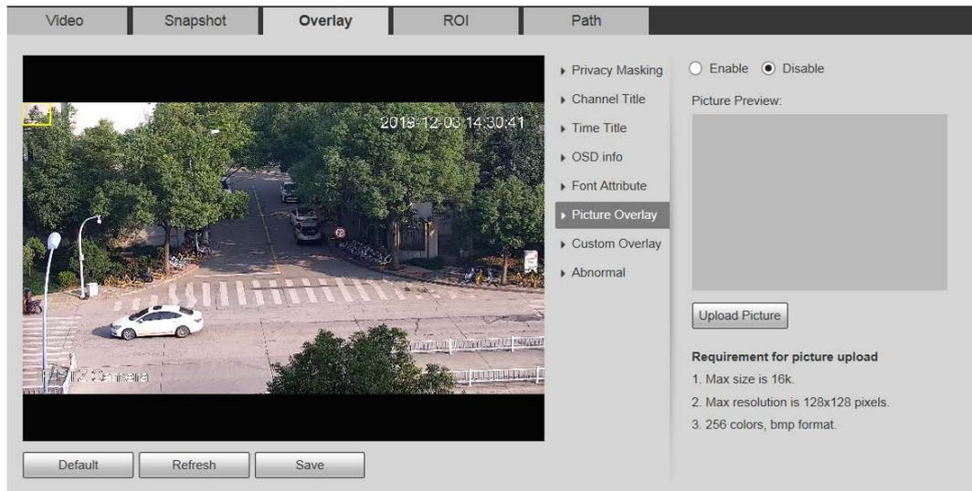
**Step 2** Select the **Enable** checkbox, click **Upload Picture**, and then select the image to be overlaid.
