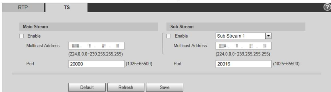
Step 2 Enable main stream or sub stream.
