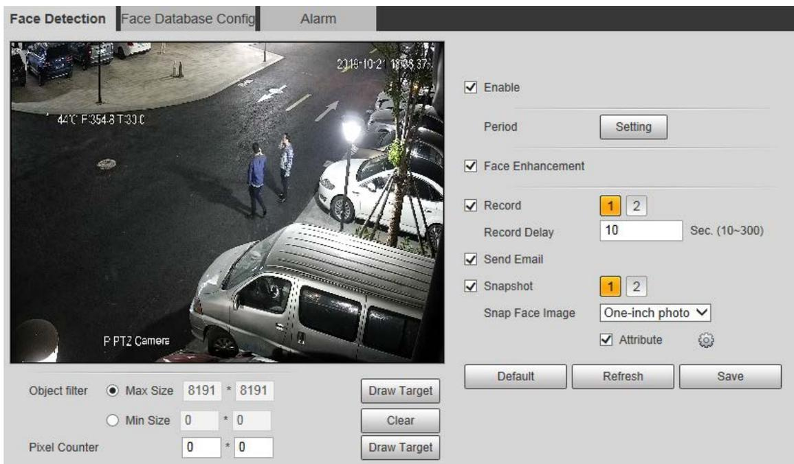
Step 2 Select **Enable** to enable the face detection function.
