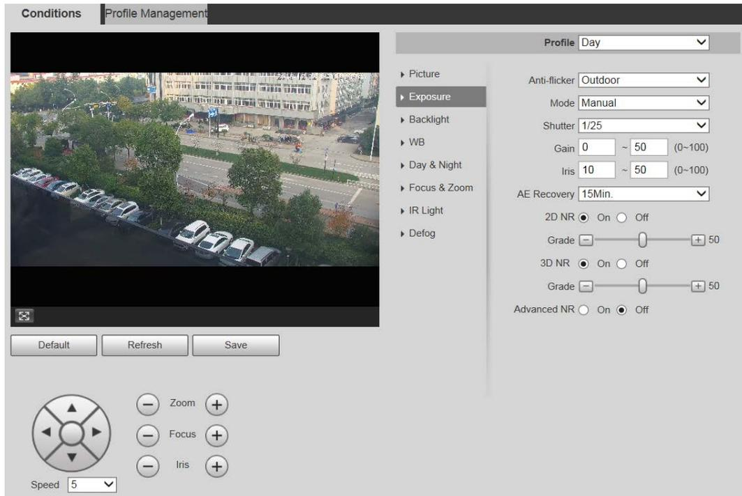
**Step 2** Configure exposure setting parameter.
