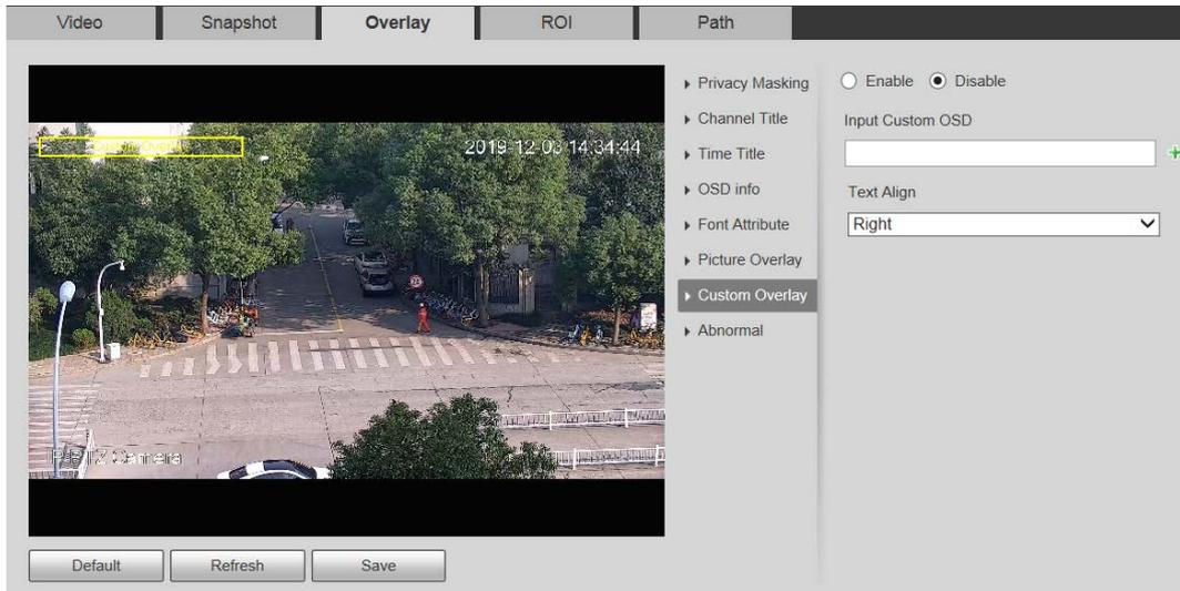
**Step 2** Select the **Enable** checkbox, and then select the text alignment.
