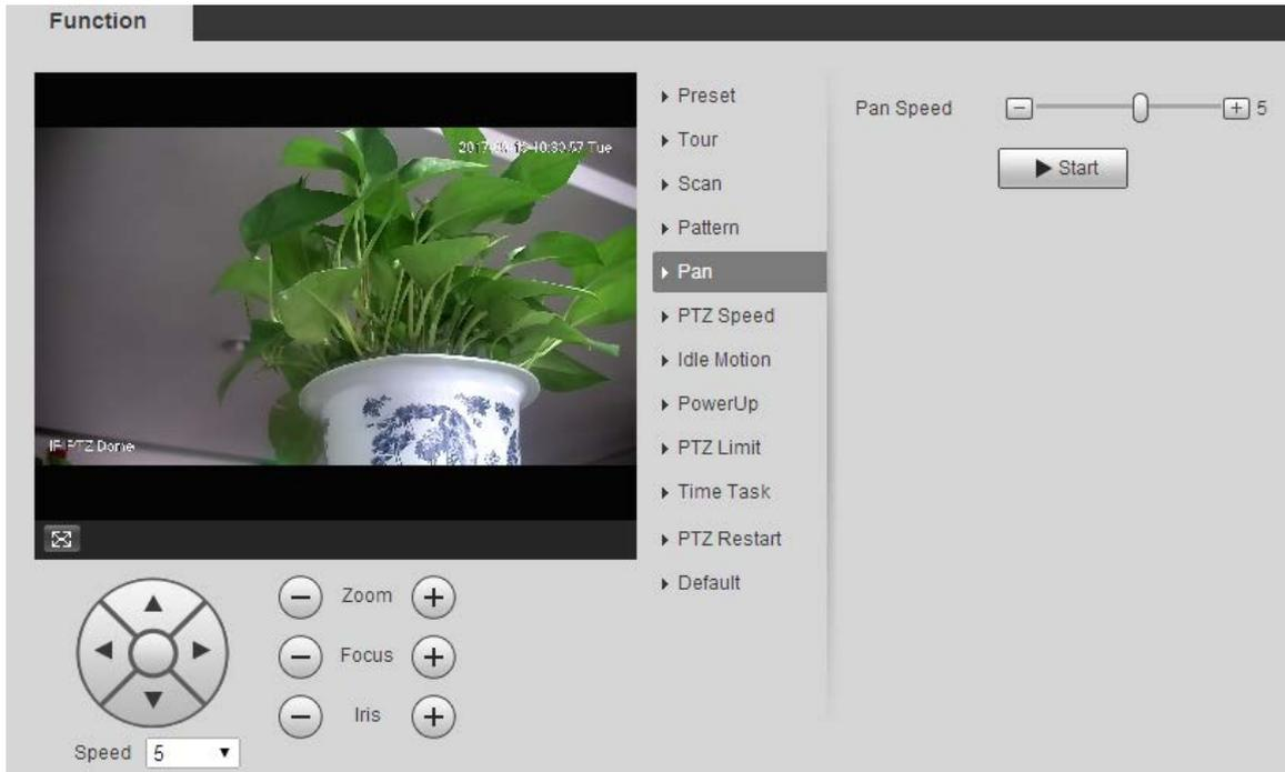
**Step 2** Drag the slider to set the **Pan Speed**.
