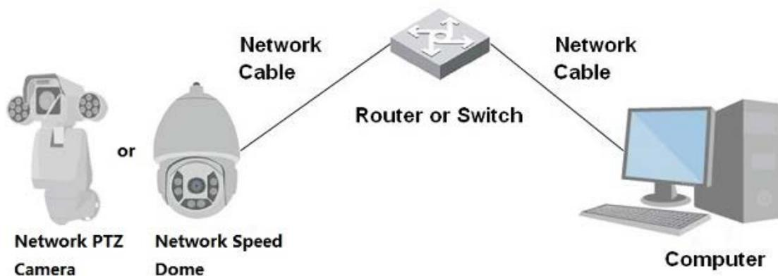
All devices have the same IP address (192.168.1.108 by default) when they are delivered out of factory. To make the Device get access to network smoothly, plan available IP segment reasonably according to practical network environment.
