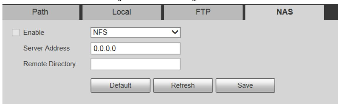
**Step 2** Configure NAS setting parameters.
