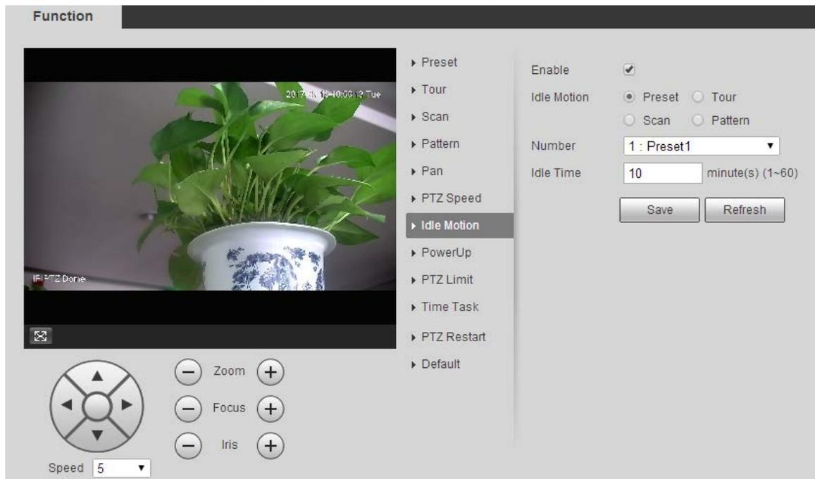
**Step 2** Select the **Enable** checkbox to enable the idle motion.
