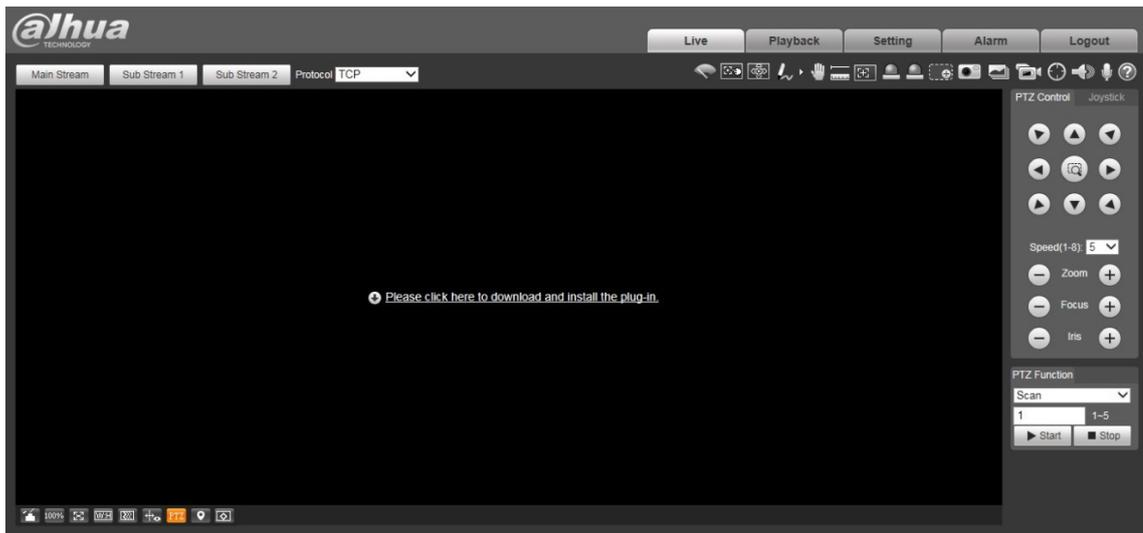
**Step 4** After the plug-in is installed, the web page will be refreshed automatically, and the video is displayed on the **Live** page.
