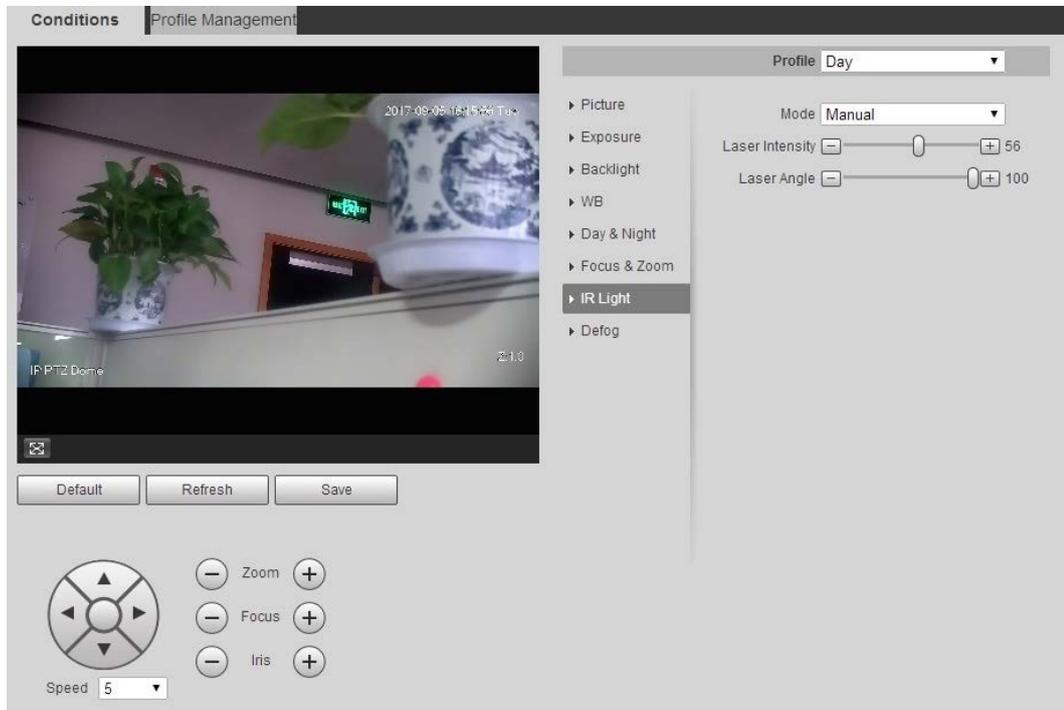
**Step 2** Configure laser light setting parameter.
