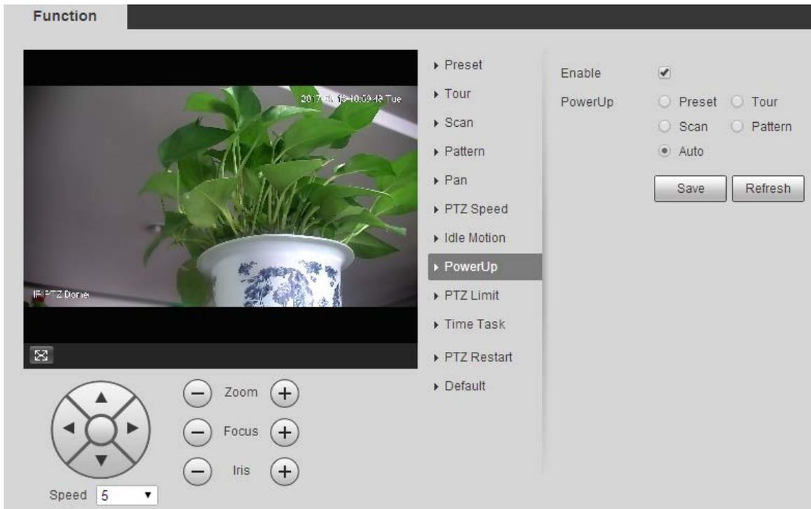
**Step 2** Select the **Enable** checkbox to enable power up motion.
