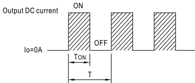
$$\text{Duty cycle(\%)} = \frac{T_{ON}}{T} \times 100\%$$
