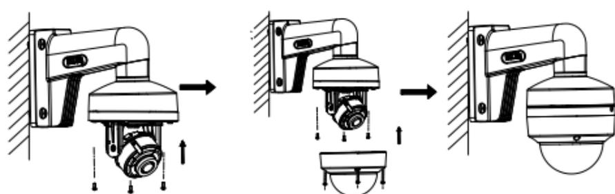
Figure 2-11 Fix the Camera to the Bracket
