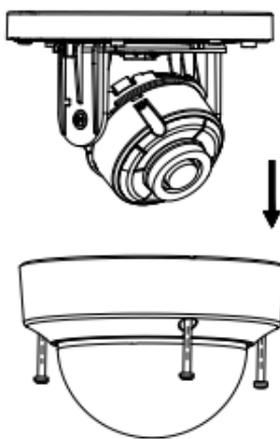
Figure 2-2 Remove the Bubble
