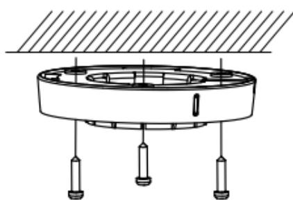
Figure 2-16 Attach the Mounting Base to the Ceiling
