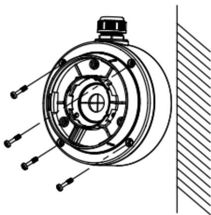
Figure 2-22 Combine the Junction Box's Cover and Body
