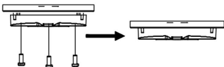
Figure 2-28 Install the Mounting Base
