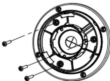
Figure 2-20 Install the Mounting Base
