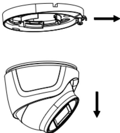
Figure 2-23 Remove the Mounting Base
