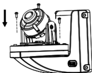
Figure 2-7 Secure the Mounting Base to the Bracket
