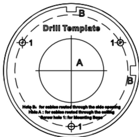
Figure 2-27 The Drill Template
