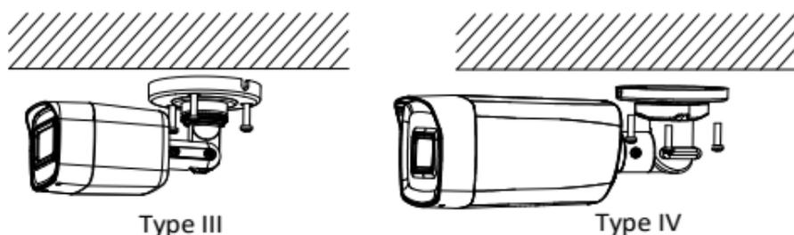
Figure 2-31 Fix the Camera to the Ceiling
