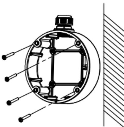
Figure 2-21 Secure the Junction Box on the Wall
