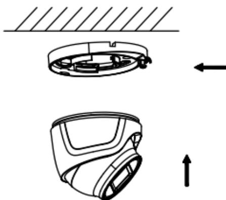
Figure 2-25 Secure the Camera
