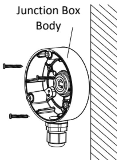
Figure 2-34 Secure the Junction Box on the Wall/Ceiling
