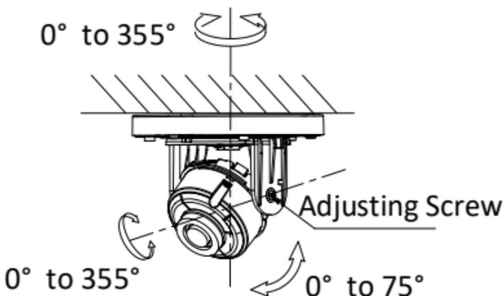
Figure 2-4 3-Axis Adjustment
