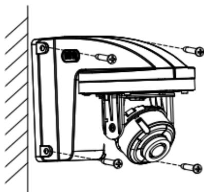
Figure 2-8 Install the Bracket on the Wall
