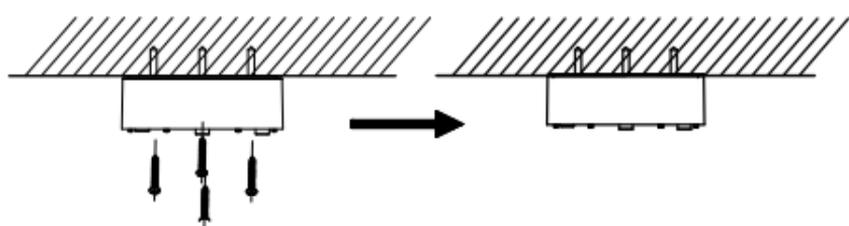
Figure 2-29 Secure the Junction Box's Body
