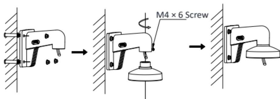
Figure 2-10 Install the Bracket
