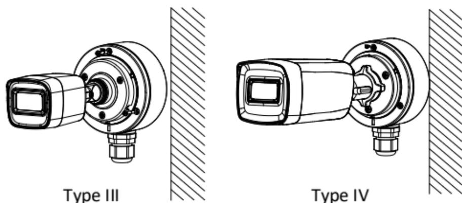
Figure 2-35 Combine the Junction Box Cover and Body
