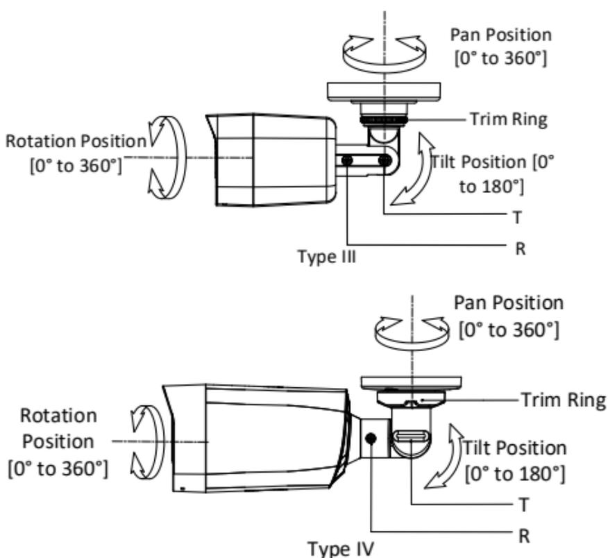
Figure 2-32 3-axis Adjustment
