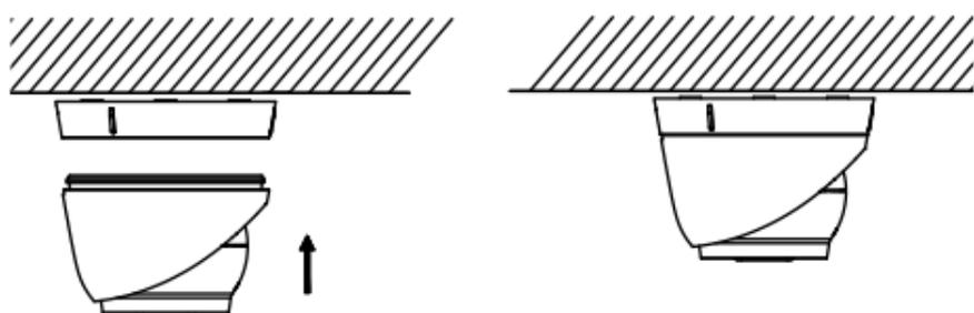
Figure 2-17 Install the Camera Back
