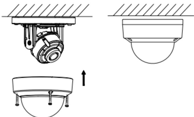
Figure 2-5 Bubble Reinstallation
