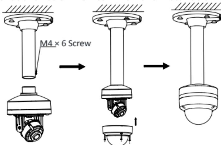
Figure 2-14 Finish Installation
