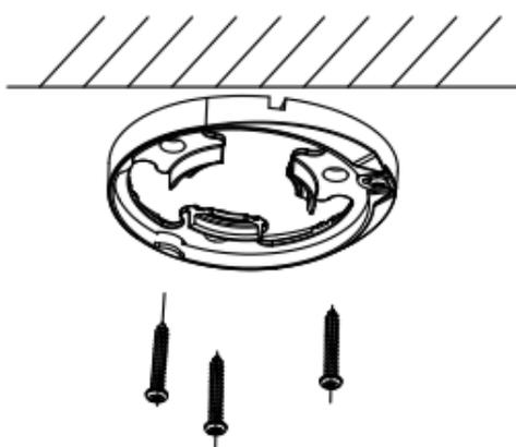
Figure 2-24 Secure the Mounting Base to the Ceiling
