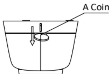
Figure 2-15 Pry the Mounting Base
