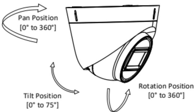
Figure 2-18 3-Axis Adjustment
