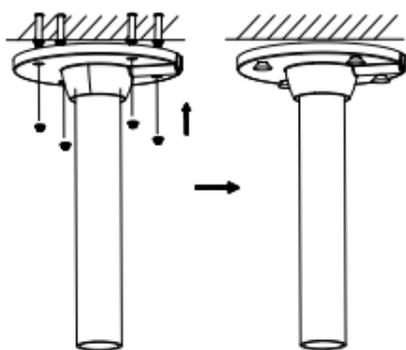
Figure 2-12 Install the Bracket to the Ceiling
