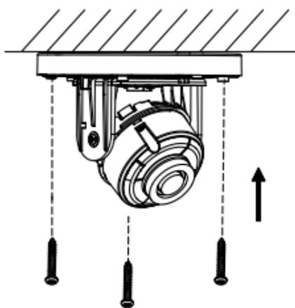
Figure 2-3 Fix the Mounting Base
