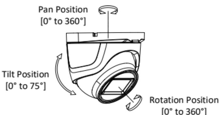
Figure 2-26 3-Axis Adjustment
